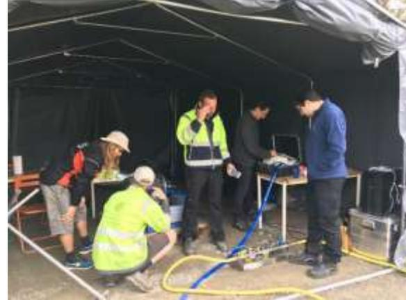
Pump-test for FFEC measurements
