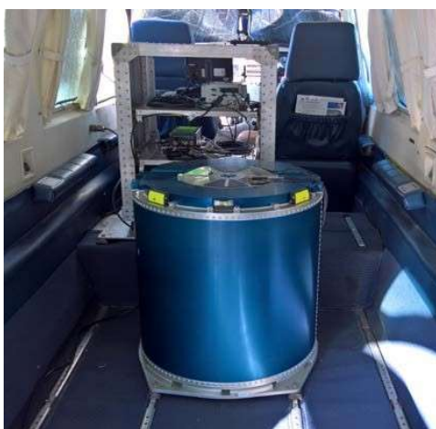
Figure A5.2: GTz (GT-3A) Gravimeter installed in a survey aircraft
