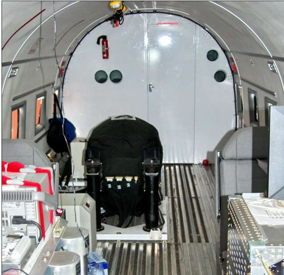
Figure A3.4: Air-FTG system installed in Basler aircraft
