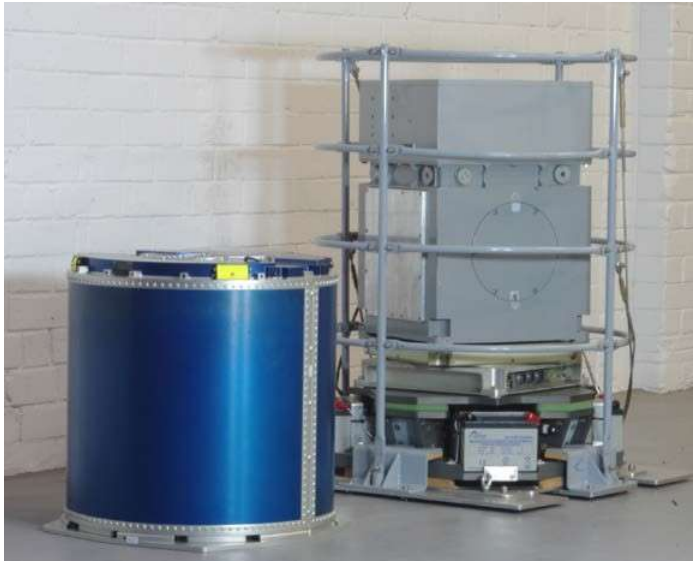
Figure A5.1: Image of GTz (left) and GT-2A (right) Airborne Gravimeters
