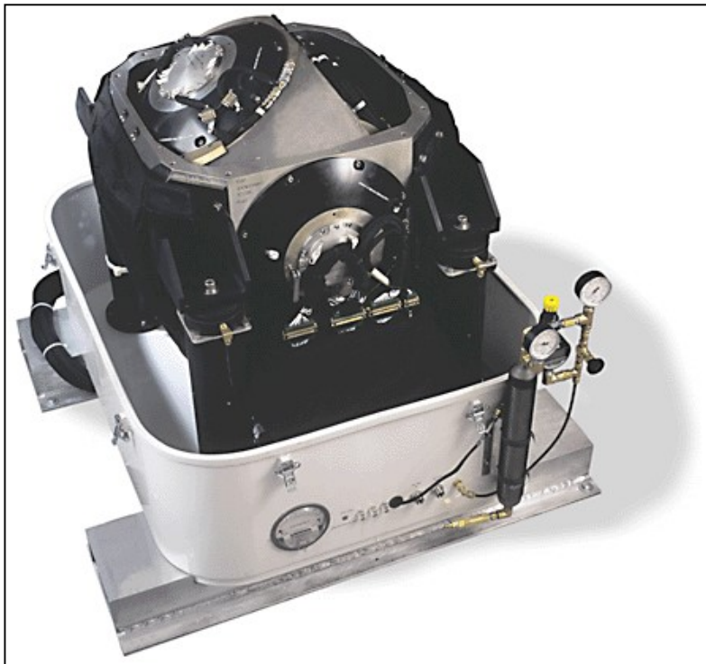
Figure A3.1: A photograph of the FTG system, with the binnacle cover removed to reveal the roll gimbal.
