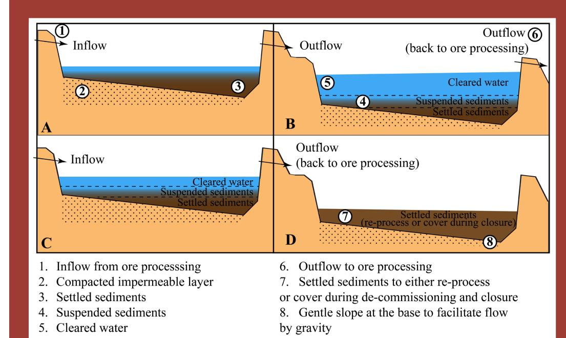
Cross section illustrating the water management in Tailing Management Facility.
