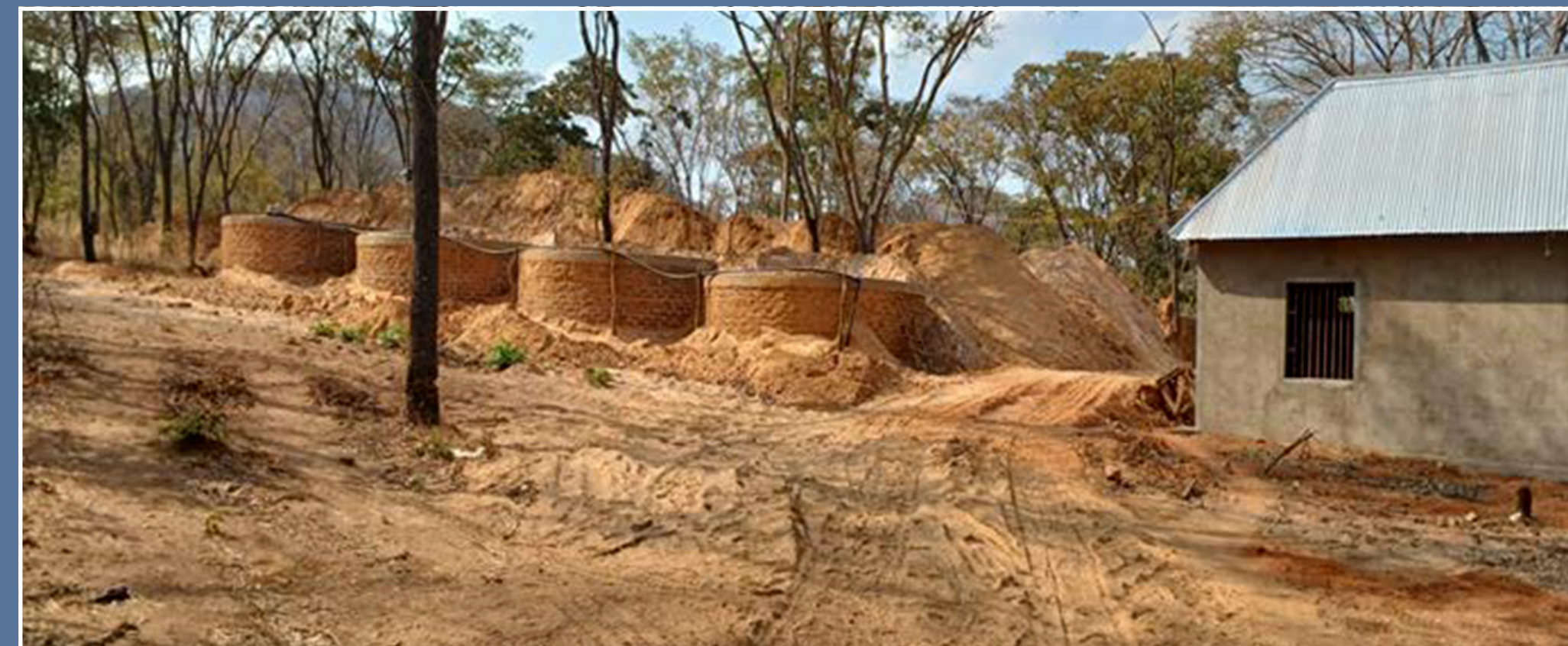
Above: Cyanide using VAT leaching plant.
